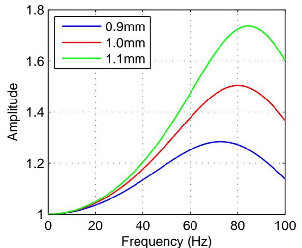
Figure 1. Amplitude response of a 750mm tube of various inner diameters.
