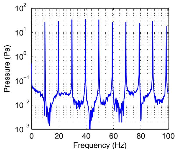
Figure 4. Spectrum of driving signal, as measured by reference transducer.
