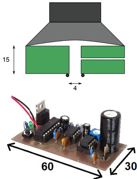
Figure 2. Dimensions of acoustic coupler (cross-section shown) and driver circuit (dimensions in mm).
