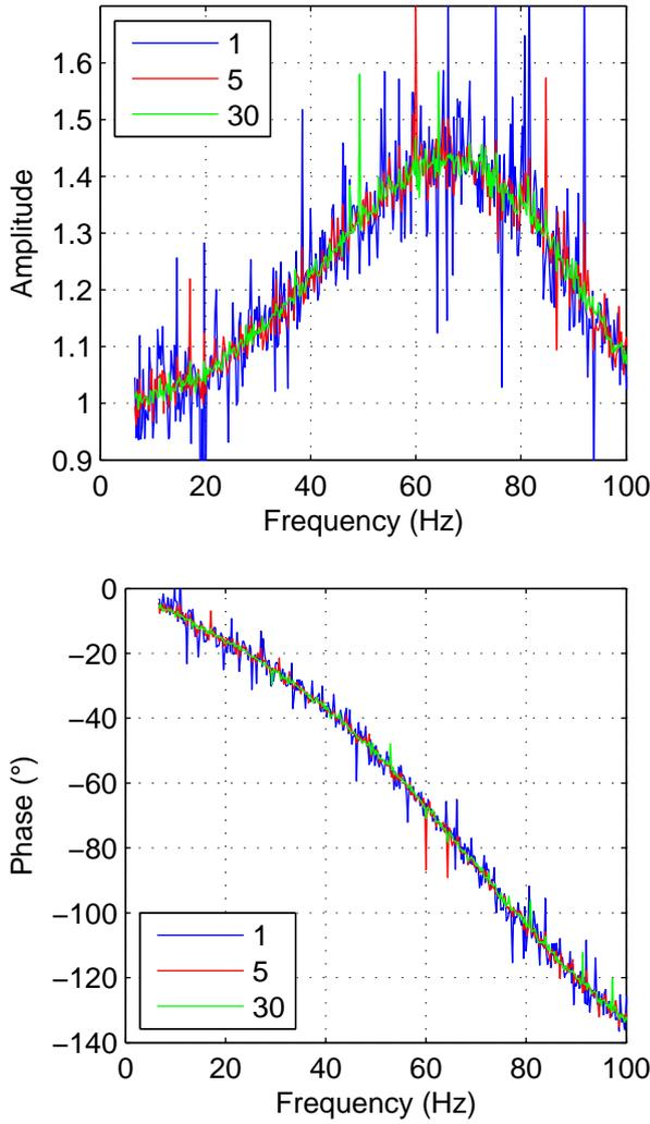
Figure 7. Amplitude and phase response of the 850mm tube obtained using the white noise method, averaging over 1, 5, and 30 realizations.
