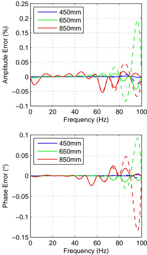
Figure 5. Amplitude and phase error resulting from cubic spline interpolation using points from 10–100Hz (---) and from 10–120Hz (—) in steps of 10Hz.
