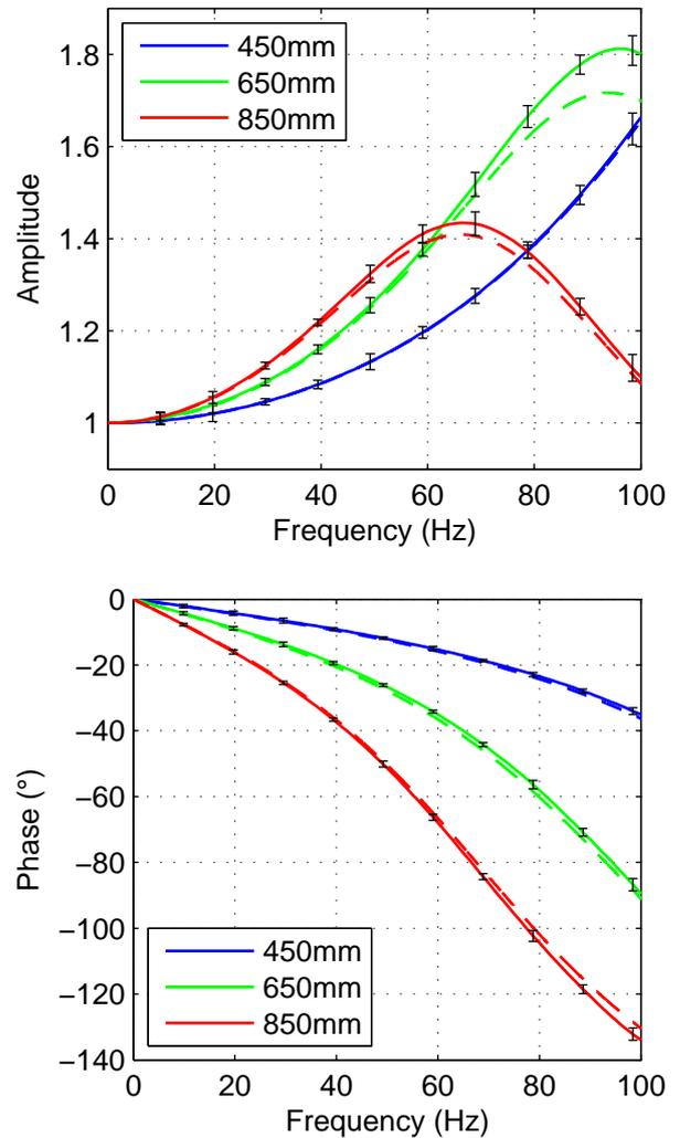
Figure 6. Amplitude and phase response as measured (—), and as calculated by the model of Bergh and Tijdenan [1] (---). Error bars show  $\pm 3\sigma$ .
