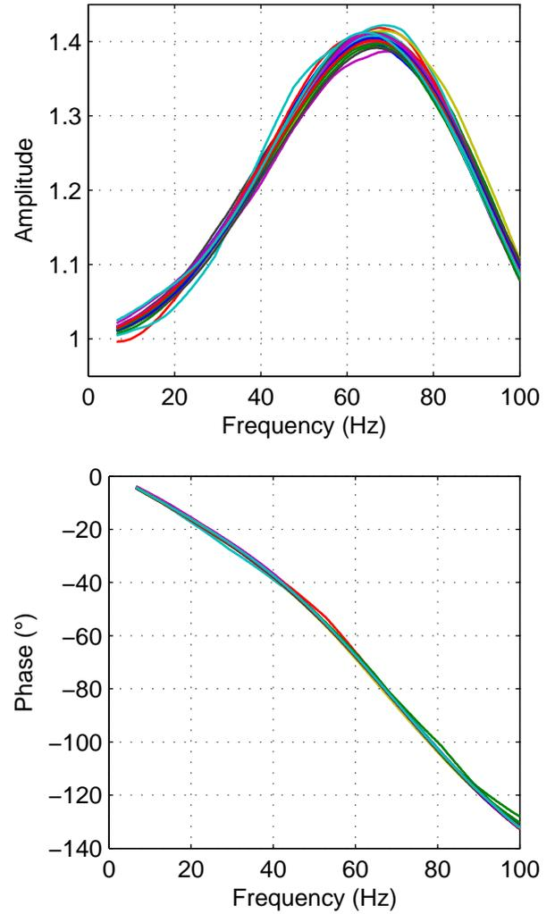
Figure 8. Amplitude and phase response obtained using the white noise method after smoothing with a moving average filter. Results of 30 repeats are plotted.
